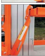
Hold down can be actuated when stabilizers are stowed.
