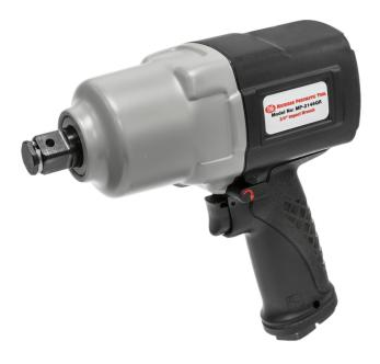
3/4" Square Drive Pistol Impact Wrench. The latest addition to the MPT product line. Features include: a lightweight composite handle, aluminum housings, twin hammers, sliding forward/reverse buttons, and an exhaust system that diverts exhaust down the handle for quiet operation and operator comfort. Ideal for rental, petro chemical and heavy industry applications.
