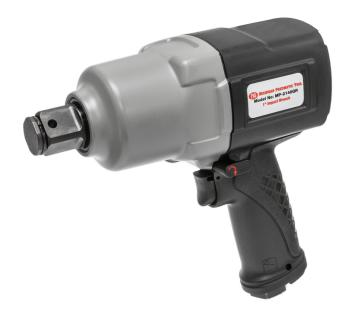
1" Square Drive Pistol Impact Wrench. The latest addition to the MPT product line. Features include: a lightweight composite handle, aluminum housings, twin hammers, sliding forward/reverse buttons, and an exhaust system that diverts exhaust down the handle for quiet operation and operator comfort. Ideal for rental, petro chemical and heavy industry applications.
