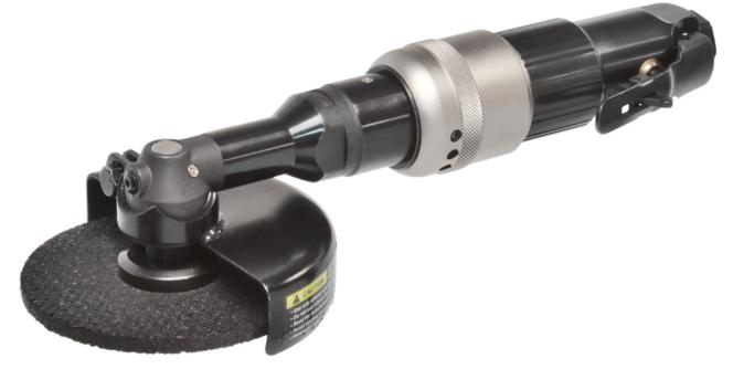
4" Type 1 Extended Angle Die Grinder. 3/8"-24 spindle. Features adjustable side exhaust and a low-profile angle head with 3 position guard for working in hard to work areas. Heavy-duty steel constructed industrial grinders for the toughest applications. Ideal for quickly removing material, deburring, chamfering in shipyards, foundry, welding, petro chemical and fabrication applications. Patented external spindle lock version also available.
