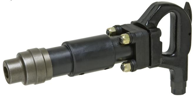
3" Stroke Outside Trigger D-Handle Chipping Hammer. Uses round shank chipper steel. The 4-bolt design helps eliminate handle breakage and allows for easy field service. Standard equipment includes chisel retainer and chisel retainer spring.
