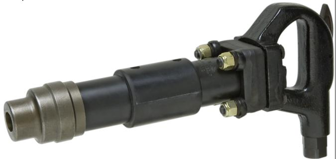
4" Stroke Outside Trigger D-Handle Chipping Hammer. Uses round shank chipper steel. The 4-bolt design helps eliminate handle breakage and allows for easy field service. Standard equipment includes chisel retainer and chisel retainer spring.
